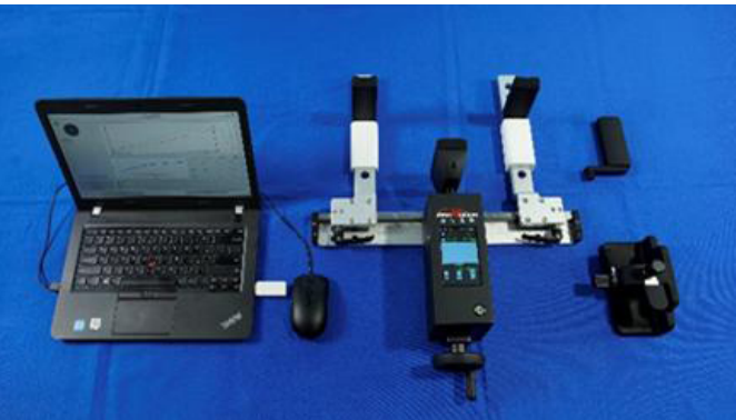
图 1 | 新型关节韧带数字体查仪照片 (逸动医学, 上海) Figure 1 | General image of novel digital arthrometer (Escape Medicine, Shanghai, China)
