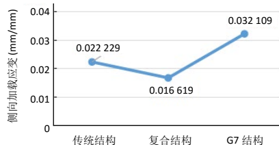
图11 | 不同结构种植体侧向静载荷应变值 Figure 11 | Lateral static load strain of implants with different structures
