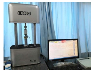
图2 | 电磁式动态力学实验系统 Figure 2 | Electromagnetic dynamic mechanical experiment system
