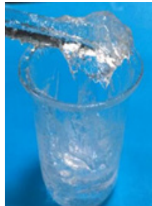
图注: 臭氧缓释水凝胶呈无色透明胶体, 具有较好的黏滞力和皮肤延展性 图 3 | 臭氧缓释水凝胶实物样品大体观 Figure 3 | General view of sample of ozone sustained-release hydrogel
