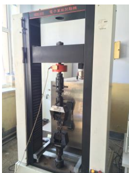
图1 坐骨神经试样拉伸实验照片 Figure 1 Tensile test photo of sciatic nerve samples
