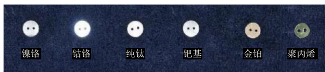
图1 六种实验试件 Figure 1 Six experimental specimens
