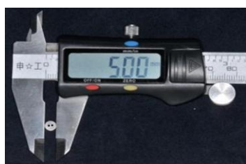
图2 试件直径 Figure 2 Diameter of the specimens
