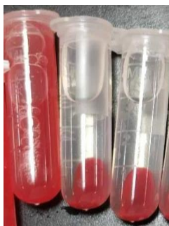
图注: 从左向右分别为含镁合金材料生理盐水浸提液的实验组、含生理盐水的阴性对照组及含蒸馏水的阳性对照组。 图5 溶血实验中各组加入稀释抗凝血温育离心后表现 Figure 5 Performance of each group in hemolysis test after adding diluted anticoagulant blood for incubation and centrifugation
