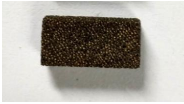
图1 多孔镁合金支架材料 Figure 1 Porous magnesium alloy scaffold materials
