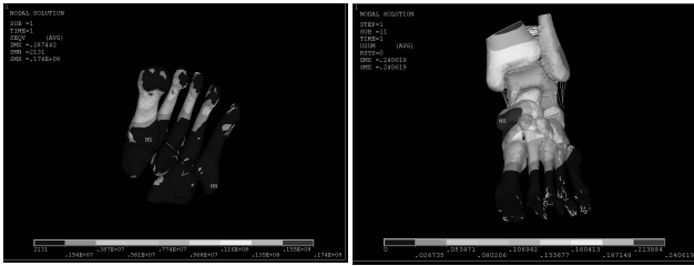
图6 在1 000 N压力的足部骨骼模型的位移矢量和 Figure 6 Displacement vector sum of the bones of foot models under 1 000 N of pressure
