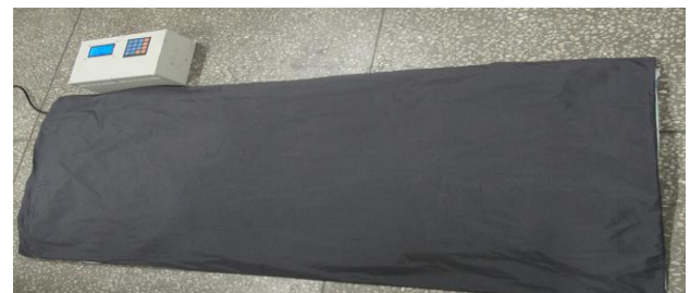
图4 医用碳纤维恒温加热垫实物图 Figure 4 Medical carbon fiber thermostatic heating pad
