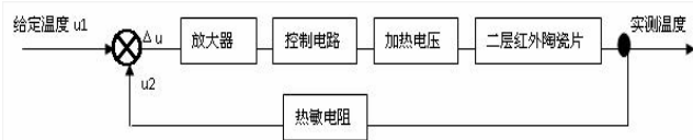
图3 温灸仪温度闭环控制系统方框图 Figure 3 Block diagram of the closed loop temperature control system
