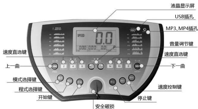
图4 某健身器材的控制界面 Figure 4 Control interface of a fitness equipment
