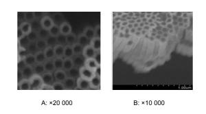
Diameter of nanotube was about 80 nm, and length of nanotube was about 2  $\mu\text{m}.$
