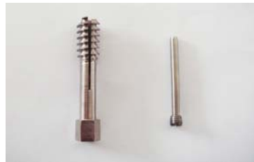
Figure 1 Hollow nail and inside plug 图1 主钉及内栓图
