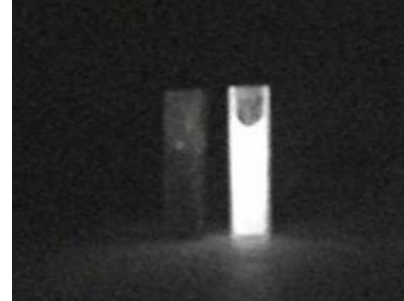
a: Colorimetric dishes image with the CCD light source distance of 25 cm
