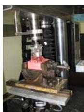
Figure 2 Loading device before titanium plate pull out
