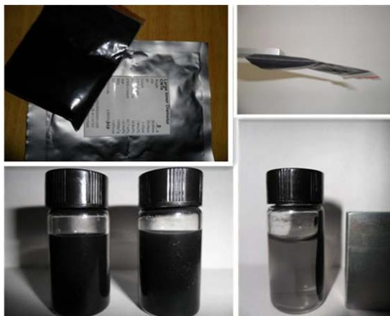
Figure 2 Suspension of magnetic carbon nanotubes
