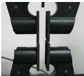
Figure 2 Air pressure holding device in the experiment 图2 实验中的空气加压夹持装置
