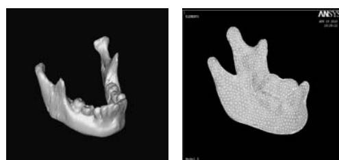
Figure 1 Three-dimensional (3-D) finite element model of the mandible
