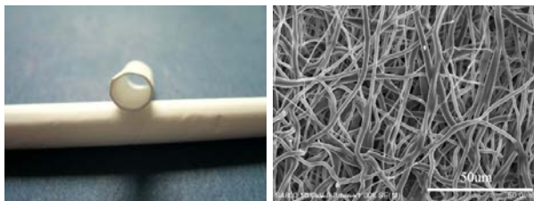
Figure 1 Polycaprolactone grafted heparin scaffold and electron micrograph 图1 聚己内酯接枝肝素人工血管支架及其电镜照片
