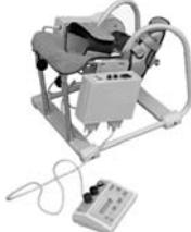
Figure 3 Intelligent ankle rehabilitation device
