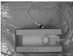
Figure 2 Self-made scanning box and the surface coil placed on the bottom 图2 自制的扫描盒及其底部安置的表面线圈
