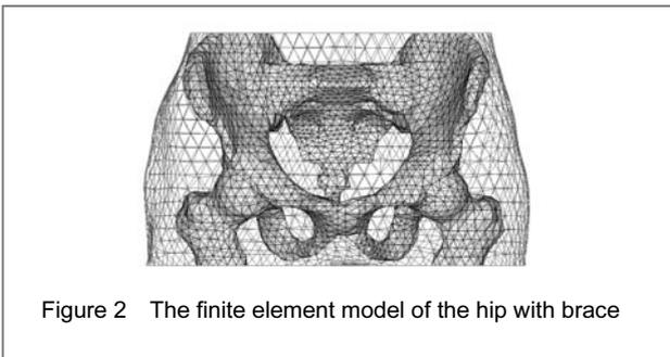
Figure 2 The finite element model of the hip with brace
