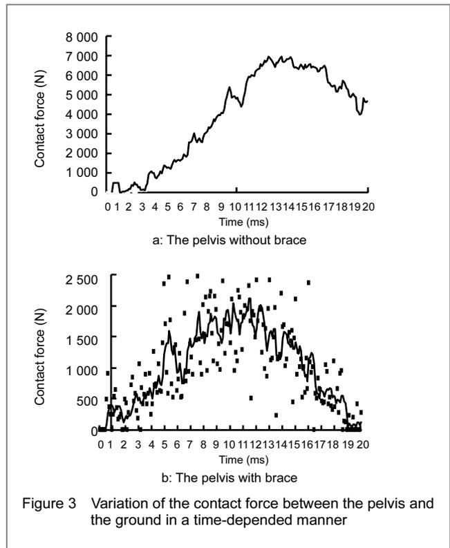
Figure 3 Variation of the contact force between the pelvis and the ground in a time-dependent manner
