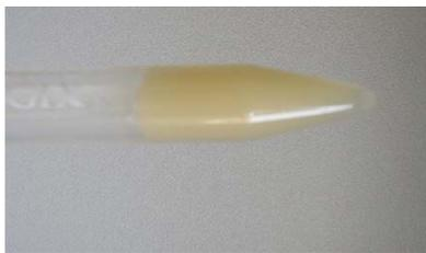
b: Thermosensitive chitosan hydrogel forms light yellow gel at 5-6 min after placing into 37 °C incubator
