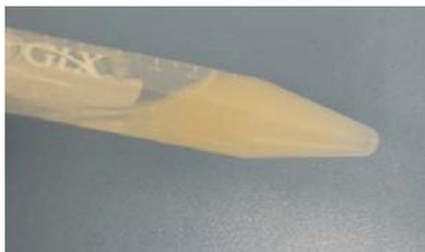
a: Thermosensitive chitosan hydrogel is light yellow liquid in room temperature
