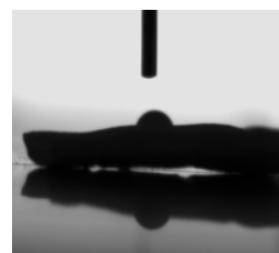
Figure 2 Contact angle following low temperature argon plasma treatment 图2 氩气低温等离子体处理后接触角
