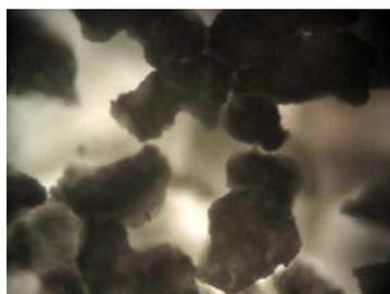
Figure 1 Nano-hydroxyapatite artificial bone under inverted microscope (×400)
