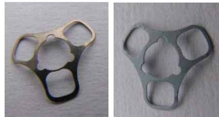
a: Pure titanium skirt b: Hydroxyapatite modified titanium skirt
