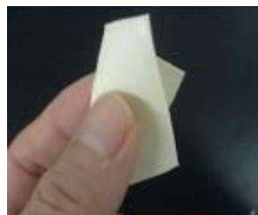
Figure 1 Appearance of scaffolds prepared by chitosan, gelatin and polyvinyl alcohol
