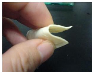
Figure 2 Appearance of scaffolds prepared by chitosan, gelatin, polyvinyl alcohol and sodium alginate
