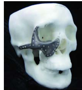
Figure 3 Titanium implant on the three-dimensional head model 图3 头颅实体模型上的数字化钛修复体
