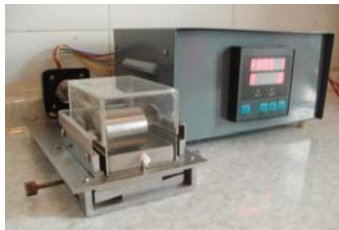
Figure 1 The photograph of the rolling depression loading device 图1 滚压加载装置的实物图
